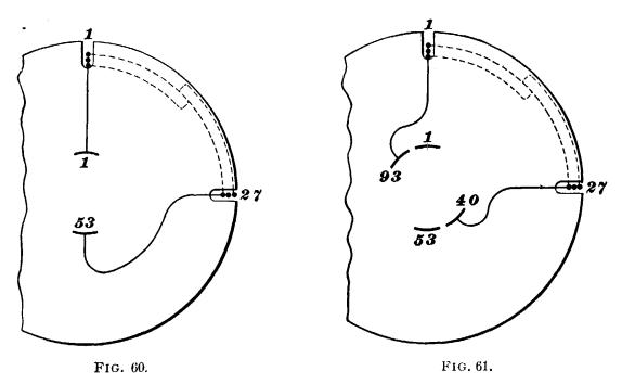
coming out of slot 27 goes half way around to bar 53. In the second case, count off a throw of 14 bars to the left from and including bar 1, which gives bar 93, the bar for the lead out of slot 1. To get the bar for the lead of the same coil out of slot 27, count off 53 to the right from bar 93, which gives 40.
