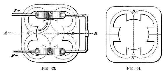
apart along the line AB. In Fig. 63, the two coils are connected correctly, and the general path of the lines of force forms the curved four-sided figure at the center. In Fig. 64, the two field coils have been left off to simplify the drawing,
