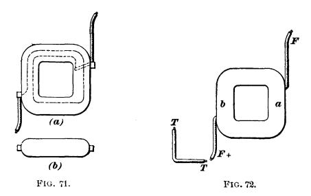
wire TT, and if it is connected to it, the current enters the coil by way of the outside end and reverses its polarity.
