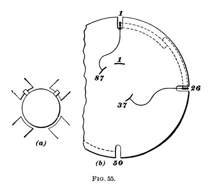
and  $\theta$  in slot 10; and so on. The short lead of coil 1 goes to bar 1 and the long lead to bar 50, as before. After one coil is installed, the others follow the same course.
