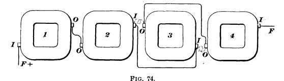
connect to I's and the O's to O's; also, that every other coil is turned end for end; this is done in order to bring together those lugs that connect together, thus avoiding a long connecting wire, which would have to be cleated up to keep it
