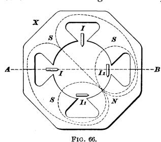
Part of the armature is, therefore, effective, and, as a matter of fact, if one coil out of four is wrongly -B connected, the car will continue to start and run on the faulty motor, but the brushes will spark badly. One wrong field coil out of four amounts to about the same thing
