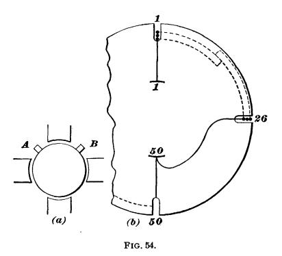
the commutator bar immediately in line with it and the long lead would go to the bar as nearly diametrically opposite as possible. This would be bar 50. The next coil would drop into slots 2 and 27 and its leads would go to bars 2 and 51. This is a rule that holds good on any armature having 99 slots and 99 coils where the four poles are on
