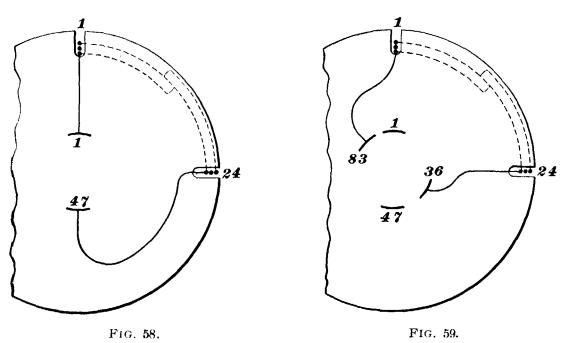
the coil drops into slots 1 and 24. In the first case, the lead out of slot 1 goes straight down to bar 1 and the lead from
