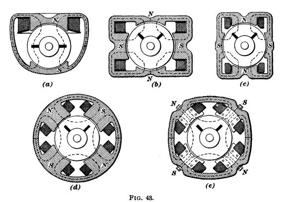
four-pole field with two field coils. (c) is the General Electric 800 (G. E. 800) motor field. It is similar to the Edison No. 14, but is turned up the other way. (d) shows the four-pole magnet frame introduced about 1891 by the Westinghouse Company in their No. 3 motor. It has four
