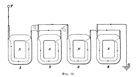
one long lead and one short one; so that if connected as shown in Fig. 69, the coils will all have the same polarity, because in each case the current goes into the coil by way
