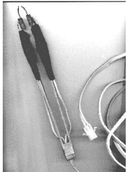
Photo 5. The tweezer electrode, made from wood pasta tongs. Note the computer power supply plug on the end of the cord.
